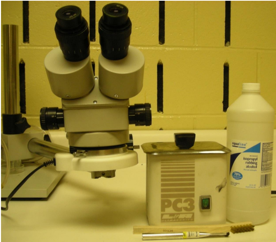
Figure 19: Stereoscope, ultrasonic bath, isopropyl alcohol, and short haired brushes.
