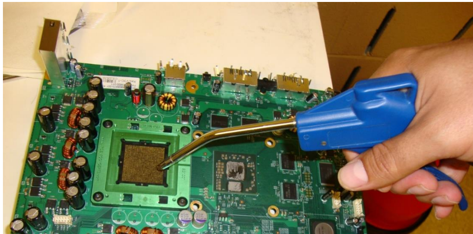
Figure 21: Socket being blown off while installed on PCB
