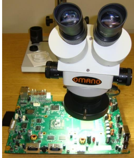
Figure 16: Examining the board under a stereomicroscope.
