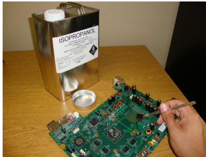
Figure 17: Cleaning the board pads with alcohol and brush.
