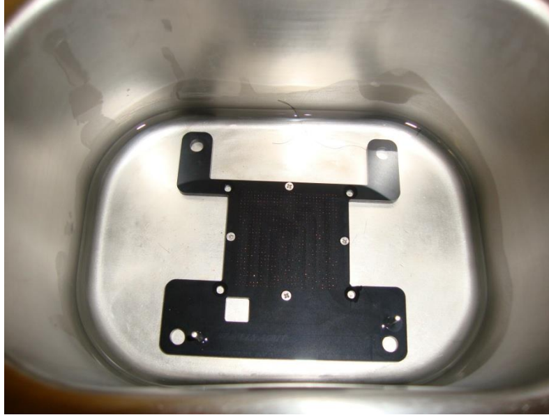
Figure 28: Interposer inside ultrasonic bath.
